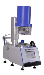
The Pneumatic 21 CFR Part 11 compliant Torque Tester is a state-of-the-art instrument designed for precise measurement and control of torque in caps, closures, and threaded components. Engineered with pneumatic holding and Electric actuation, it ensures consistent, operator-independent testing with minimal human error.
